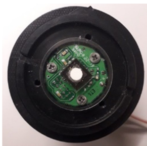
Fig. 4. Photo of a 0.5 mm thick specimen coupled to the SiPM.
