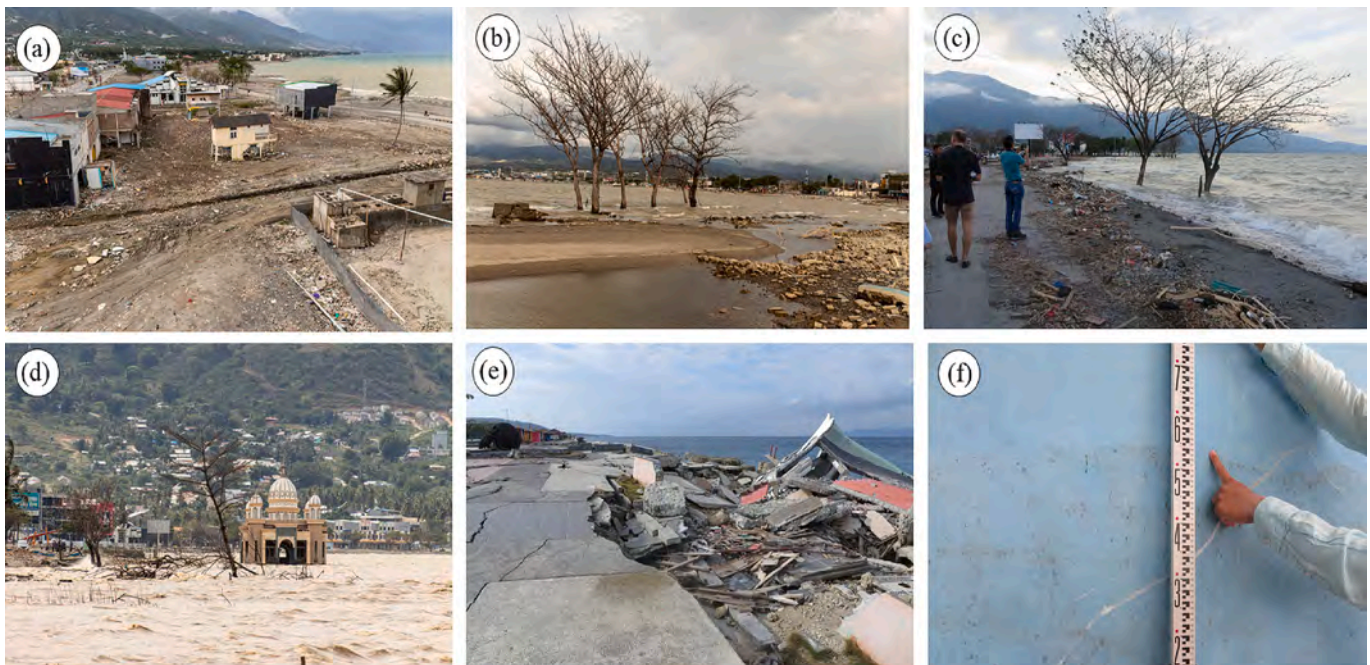
Fig. 8. Field photographs showing the tsunami inundation around the (a) Palu city, (b) Donggala city, (c) Pantaloan, (d) Apung Palu Mosque, Palu, (e) damaged pavement due to tsunami in Buluri, (f) tsunami inundation mark in building wall in Silae.
