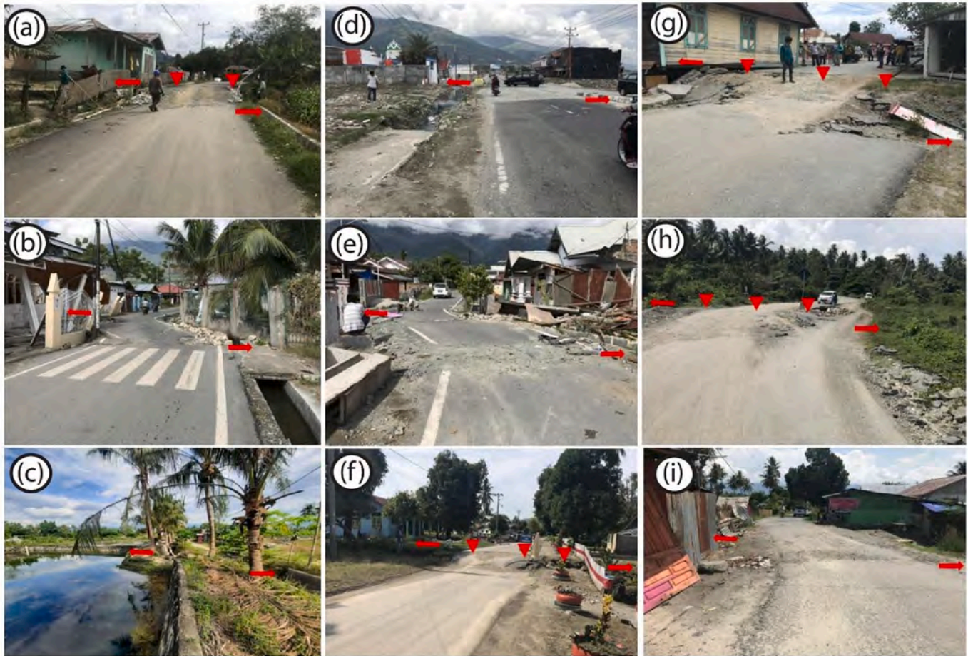
Fig. 7. Field photographs showing evidences for surface rupture of 28th September 2018 Mw 7.5 Sulawesi earthquake at (a) Amal (H = 40 cm; V = 7 cm); (b) Cembra I (H = 310 cm; V = 30 cm); (c) Rapadende (H = 420 cm; V = 20 cm); (d) Diponegoro (H = 240 cm; V = 27 cm); (e) Camera II (H = 340 cm; V = 20 cm); (f) Pakuli (H = 350 cm; V = 29 cm); (g) Dolobarat (H = 350 cm; V = 29 cm); (h) Balise-Biromaru (H = 370 cm; V = 40 cm); (i) Manunggal-Balise (H = 390 cm; V = 21 cm). The red arrow shows the sense of horizontal movement. (H=Horizontal displacement; and V=Vertical displacement of the ground surface). (For interpretation of the references to color in this figure legend, the reader is referred to the web version of this article).
