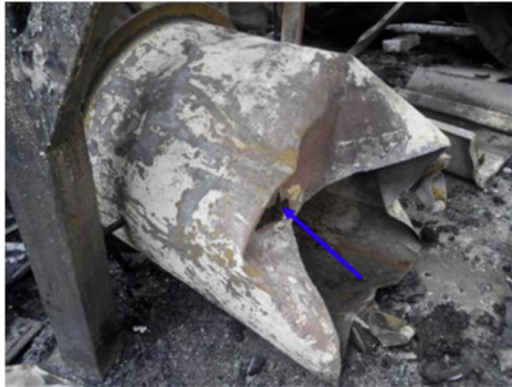
Figure 2.11: Picture of the dust collecting barrel of the #1 filter (Source: Eckhoff R., 2015)
