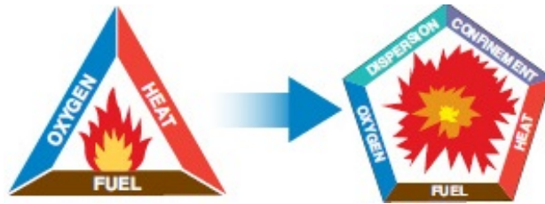
Figure 2.1: From the classic fire triangle to the dust explosion pentagon (Source: Occupational Safety and Health Administration)
