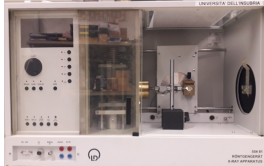
Figure 5.7: X-ray apparatus with Molybdenum anode by LD Didactic (model 554 801). The tube voltage and tube current can range from 0 to 35 kV and from 0 to 1 mA respectively.
