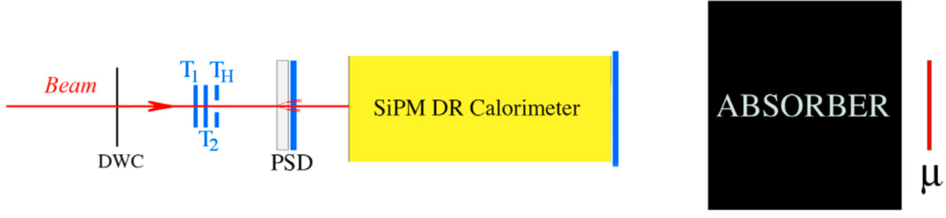
Fig. 6.1: Schematic layout of the experimental set-up (not to size). Shown are the delayed wire chamber (DWC), the trigger counters (TC), the pre-shower detector (PSD), the DR calorimeter and the muon counter ( \mu ) used in the beam test [1].
