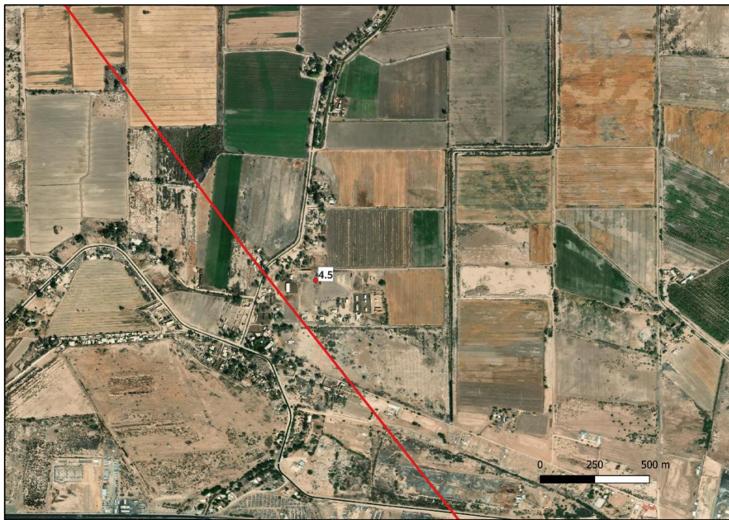
Figure 2.1 Detail of the rupture map for the 1940 Imperial Valley earthquake (California). Example of a measurement point not in accurate spatial association with the corresponding rupture trace. The point, whose label indicates the amount of recorded displacement (in meters), is located more than 100 m away from the rupture trace to which it should refer. Red line represents principal (primary) fault rupture trace, red dot indicates measurement point.
