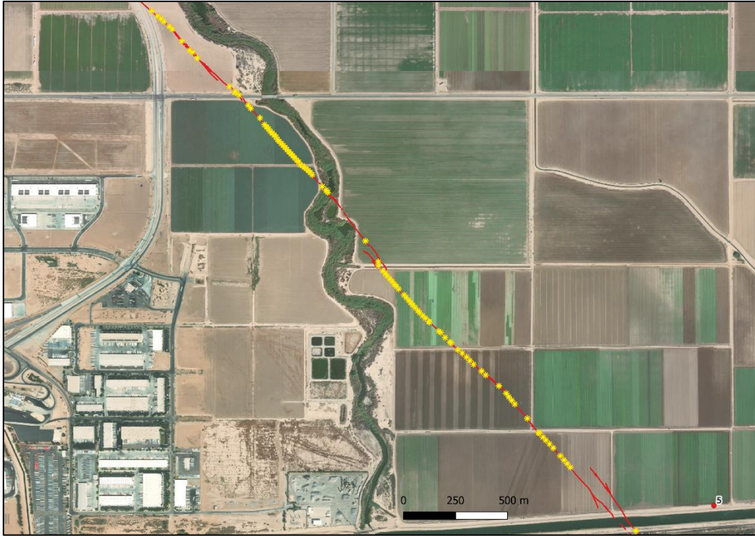
Figure 3.3 Detail along the rupture trace of the Imperial Valley earthquake (May 18, 1940, M_w \approx 7 ), showing the measurement points positioned along the fault. Points marked with yellow stars indicate the entries flagged with cumulative rank.
