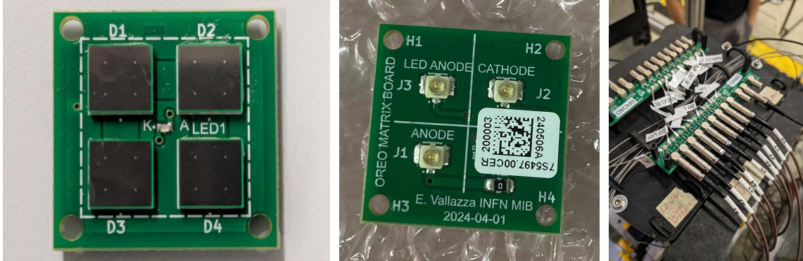
Figure 3.10: (left and center) Photo of a MPPC matrix used for the OREO readout (front and back). (right) Photo of the readout board.
