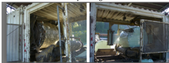
Fig. 1. HDPE plastic net wrapping (L); LDPE film protection (R)
