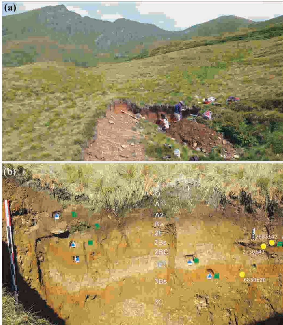
Figure 2. (a) General view of the study area during the opening of the test trench. In the foreground, the high portion of the deep-seated gravitational slope deformation (DSGSD) is visible to the right; the DSGSD is broken downslope to the left by a morphological trench associated with a counterscarp. In the background, the peak of Mt. Pizzo di Gino and its southern slope are visible to the left. (b) Picture of the investigated polycyclic soil sequence indicating the position of soil horizons and samples for analyses (squares: blocks for thin sections; triangles: samples for chemical–physical analyses; dots: samples for radiocarbon dating).
