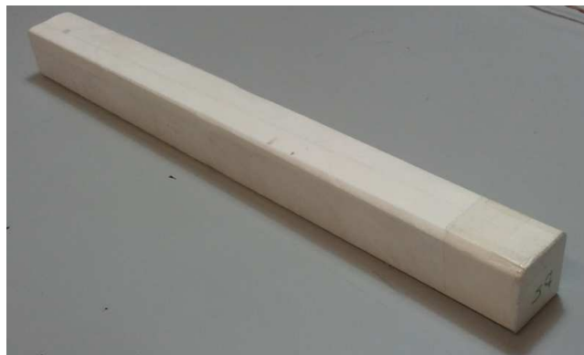
Figure 6.2: Picture of the PbWO 4 crystal wrapped in the Tyvek sheet.
