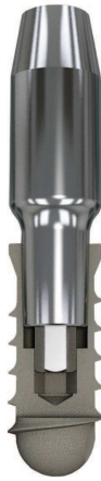
Fig. 1. Schematic representation of the implant-abutment connection of the Exacone Implant System® (Leone, Florence, Italy). The implant-abutment connection features a self-locking Morse taper combined with an internal hexagon for the repositioning of the abutment. The Morse taper presents a taper angle of 1.5°.
