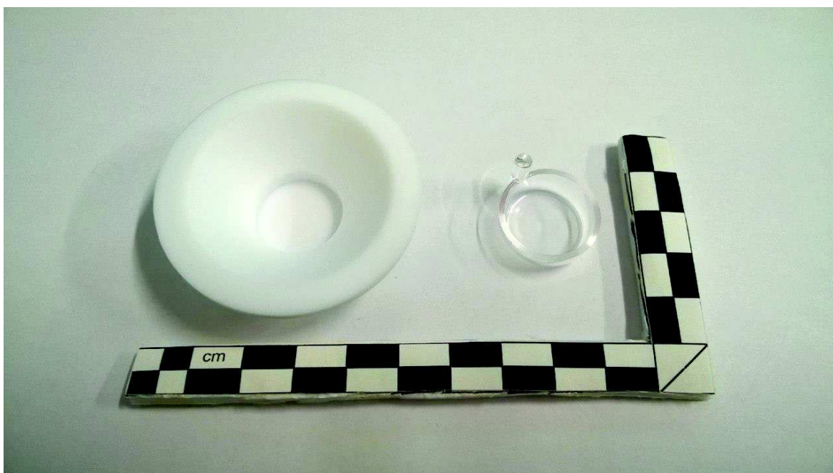
Figure 3.8 - Comparison between the cell made in PTFE and the new cell made in quartz.
