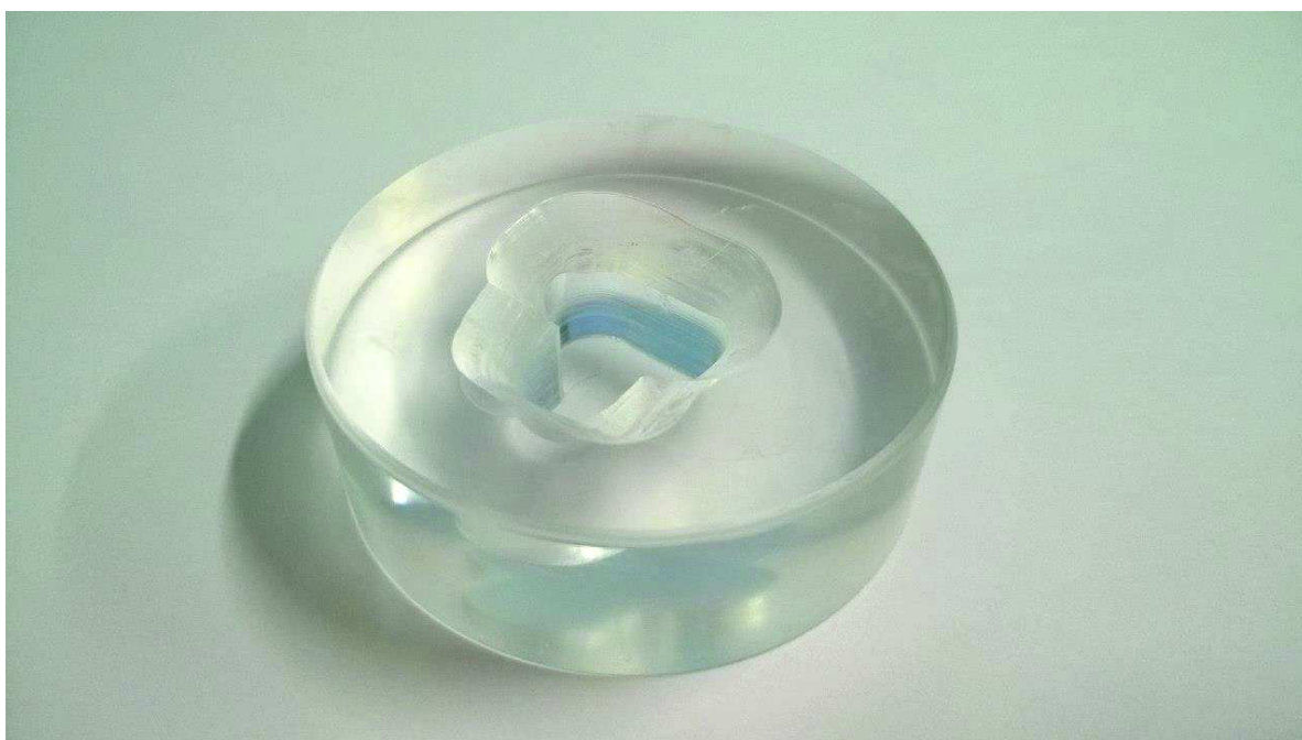
Figure 3.2 – Bottom part of the first prototype photo. This portion was realized in polystyrene.
