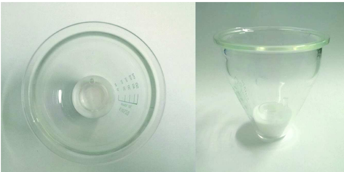
Figure 3.10 - Aspect of the new cell system using the new PTFE stand and the quartz cell.
