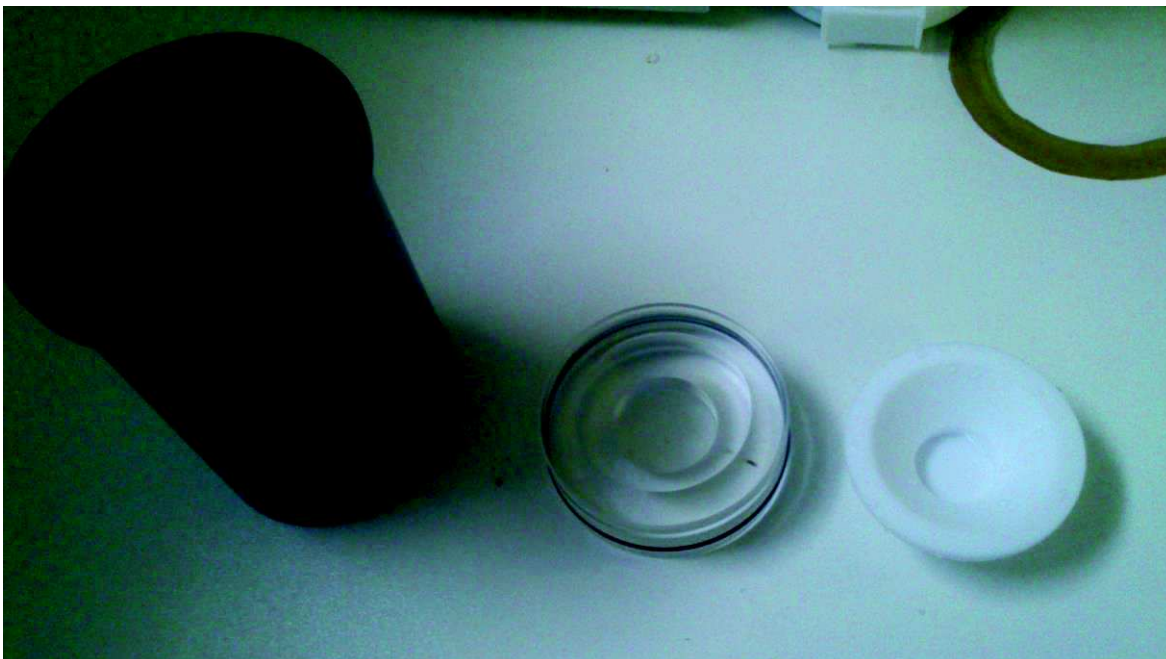
Figure 3.6 – Photo of the second prototype. The black support was unchanged, the bottom part is formed by two pieces now: a support in polystyrene and the actual cell in PTFE.
