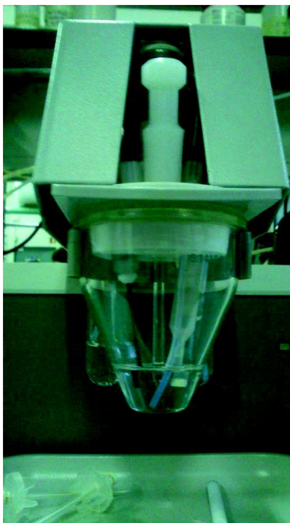
Figure 3.1 – Photo of standard configuration of the voltammetric system (Metrohm 757 VA)
