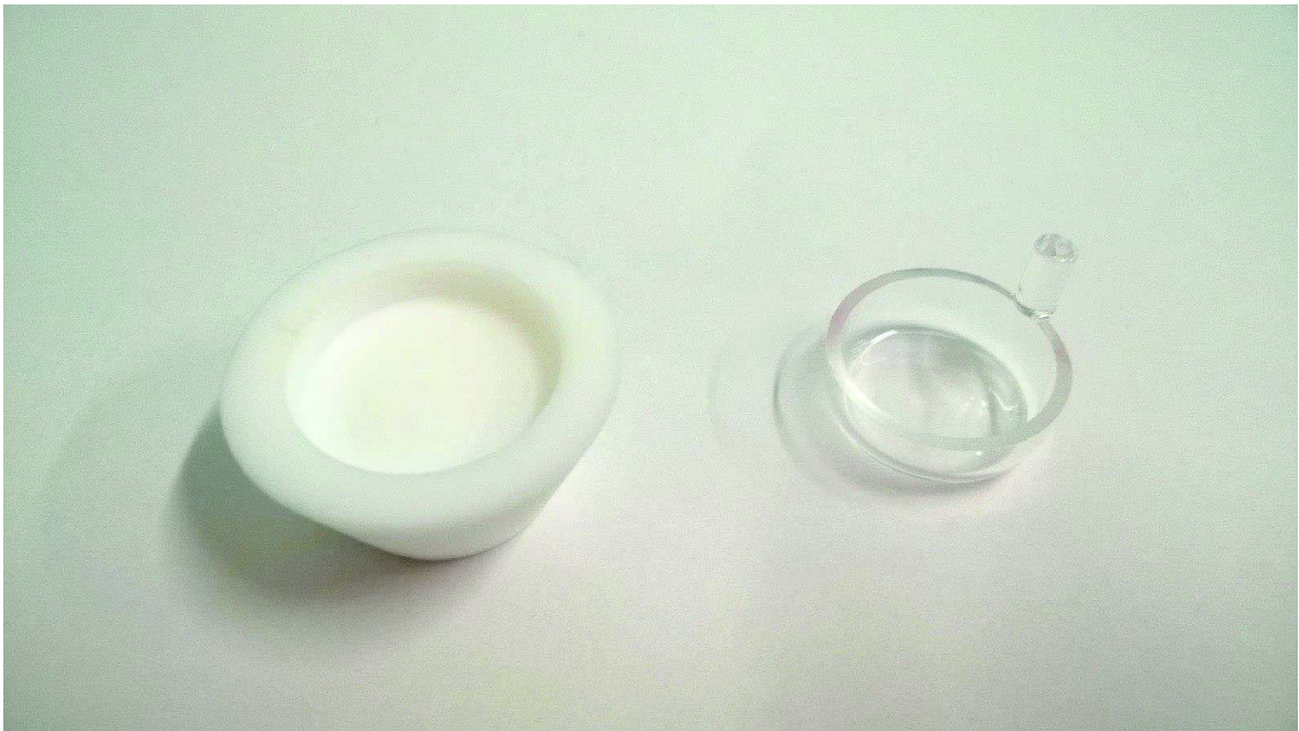
Figure 3.9 - Photo of a PTFE cell stand and quartz cell. The stand was necessary in order to use the standard glass cell available from Metrohm.
