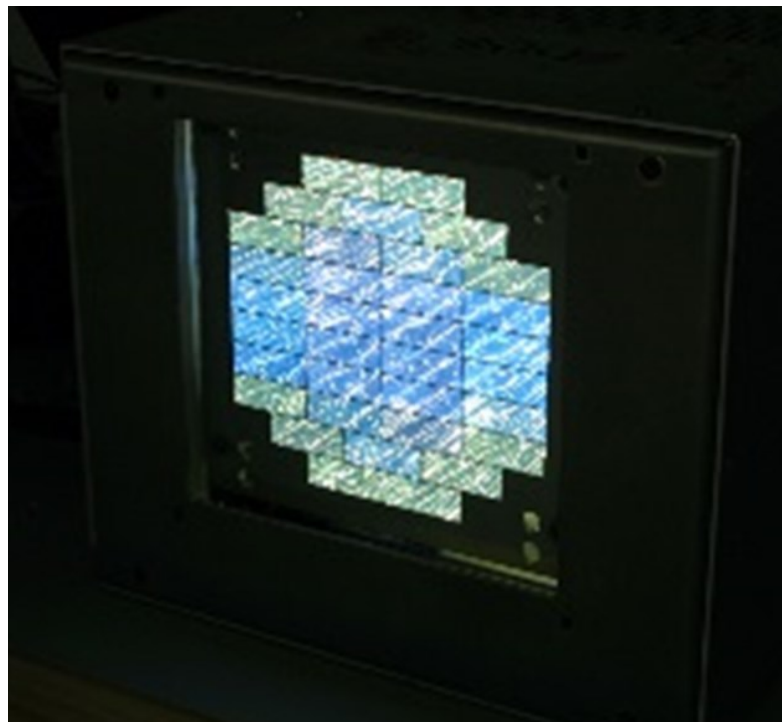
Figure 48 - Scattering from the reflector, making visible color disuniformity of DispE prototype
