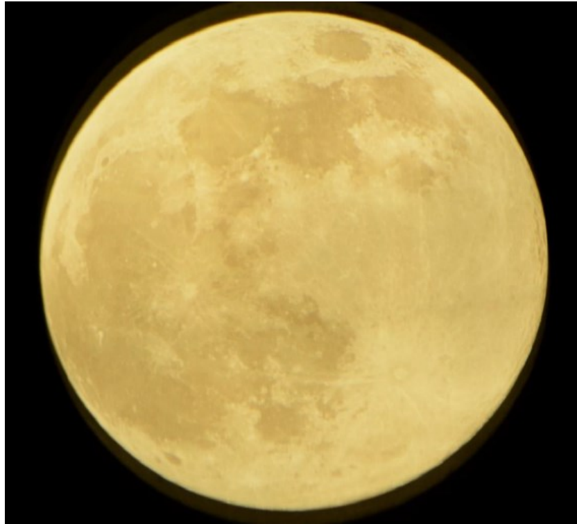
Figure 100 - Artificial moon visible face In this picture are also visible top and bottom edges reflected due to the thickness of the CoeLux panel (Fresnel reflection)
