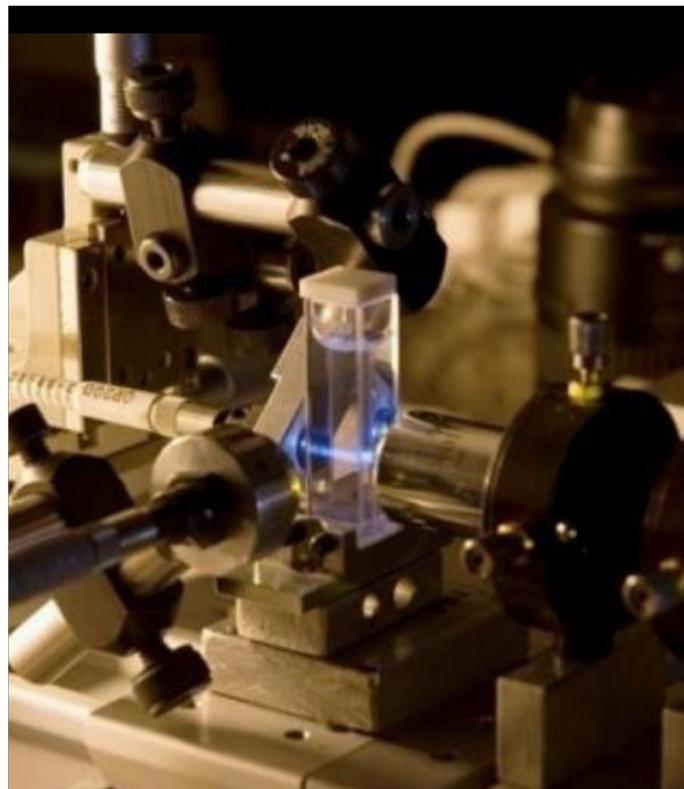
Figure 4 - Light scattering experiment in laboratory
