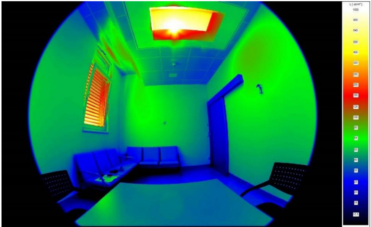
Figure 111 - False colors image (Luminance) of the sceneview from the patient seat in Hall in Tirol clinic
