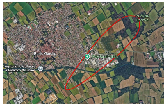
(c) Predicted impact area under stability class 2F calculated with ADAM.
