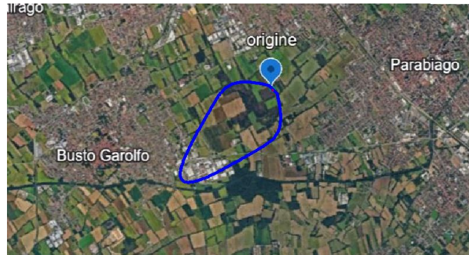
(a) Predicted impact area under stability class 2F calculated with PHAST.
