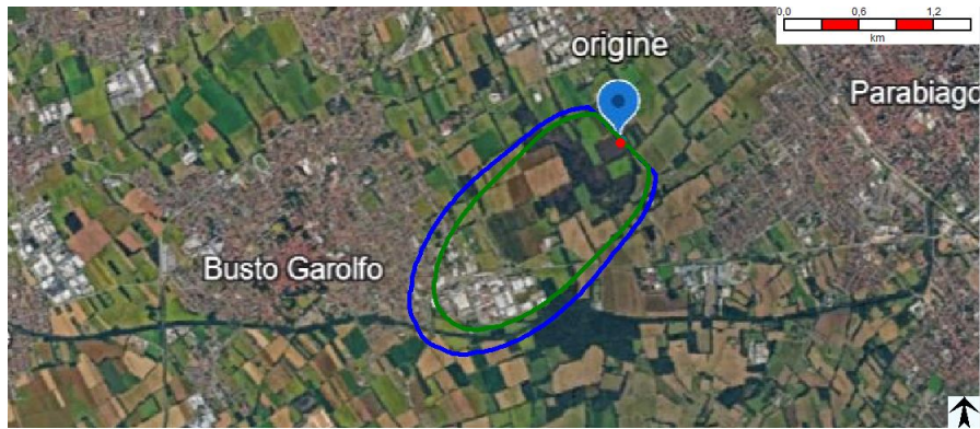
(a) Predicted impact area under stability class 2F calculated with PHAST.
