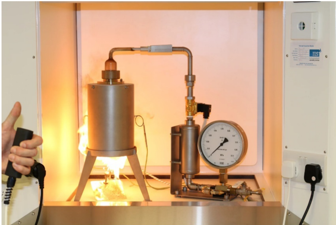
Figure 3.32: Vertical Godbert–Greenwald (G–G) furnace. Source: Sigma-HSE, “Dust and Powder Testing,” https://sigma-hse.com/testing/dust-powder-testing-
