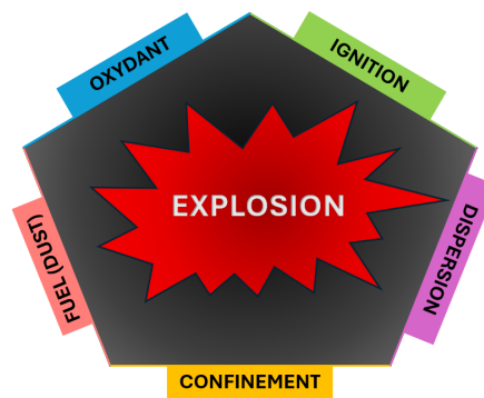
Figure 3.27: Explosion pentagon for dust explosions.
