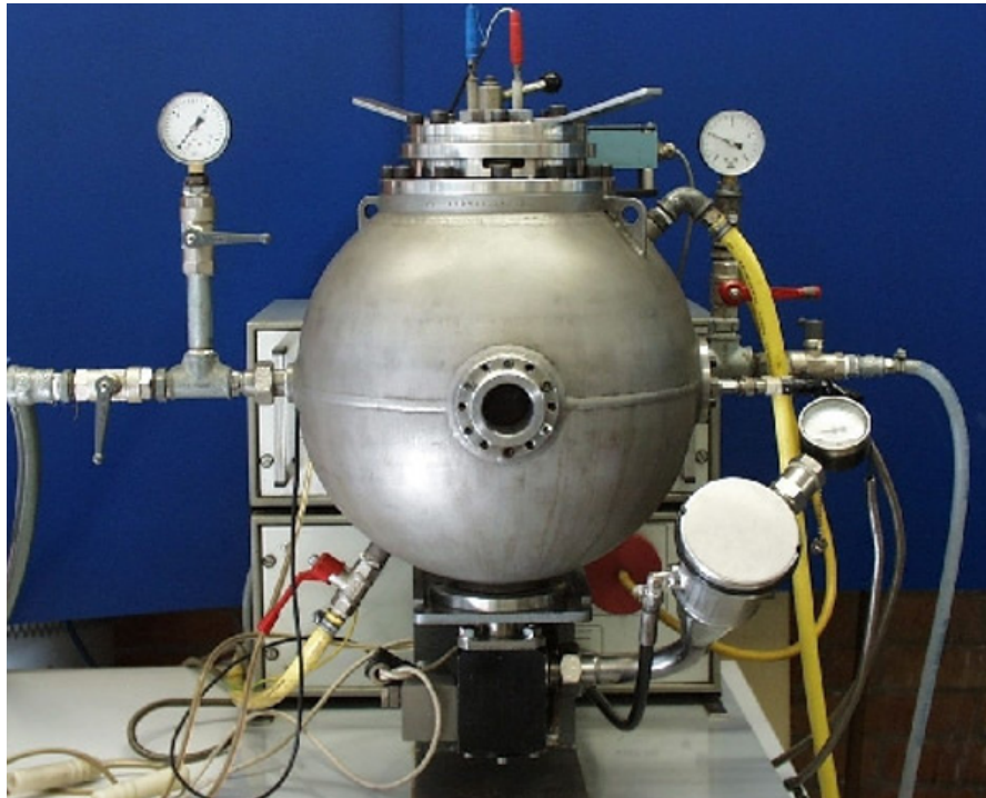
Figure 3.30: 20-L Sphere apparatus. Source: Adinex, Dust Explosion Testing – 20 L Sphere. https://www.adinex.be/en/stofexplosies/20-liter-bol/ .
