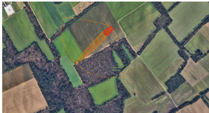
(b) Predicted impact area under stability class 2F calculated with ALOHA.
