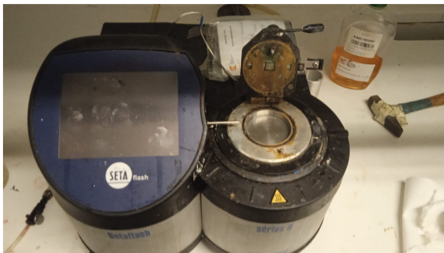
Figure 3.25: Pensky – Martens closed cup apparatus used for flash point determination.
