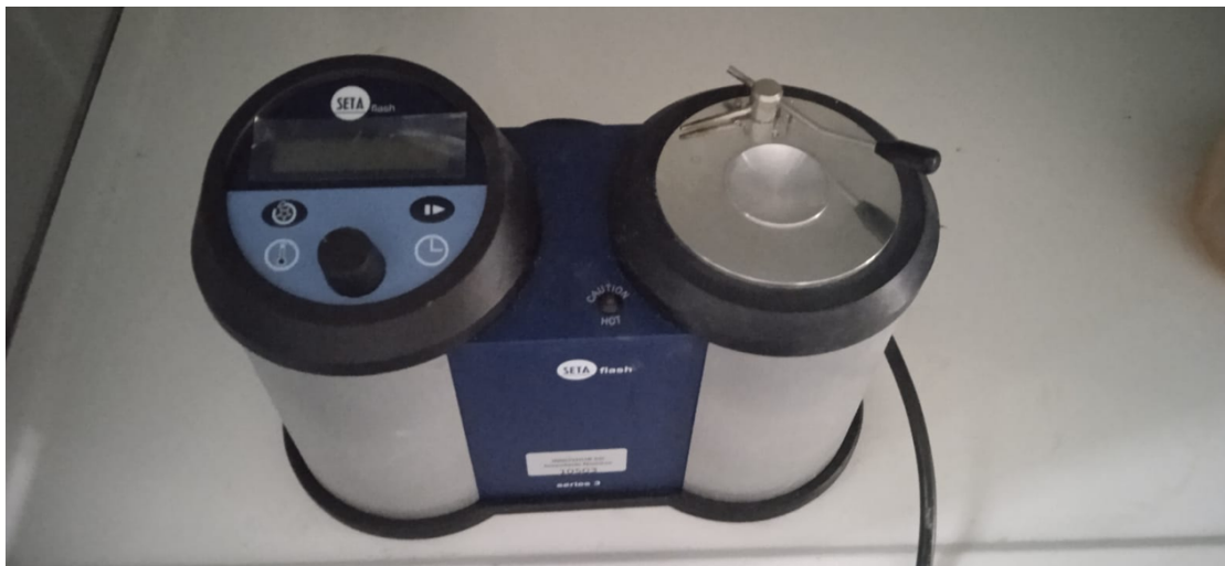
Figure 3.24: Determination of the flash point temperature using the open cup method.
