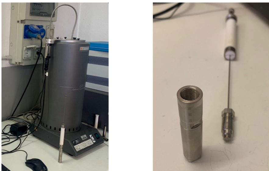
Figure 3.10: Schematic representation of the 3D sensor of a C80 calorimeter.
