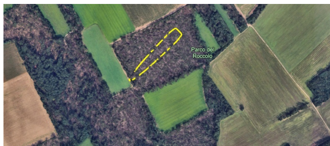
(c) Predicted impact area under stability class 2F calculated with ADAM.
